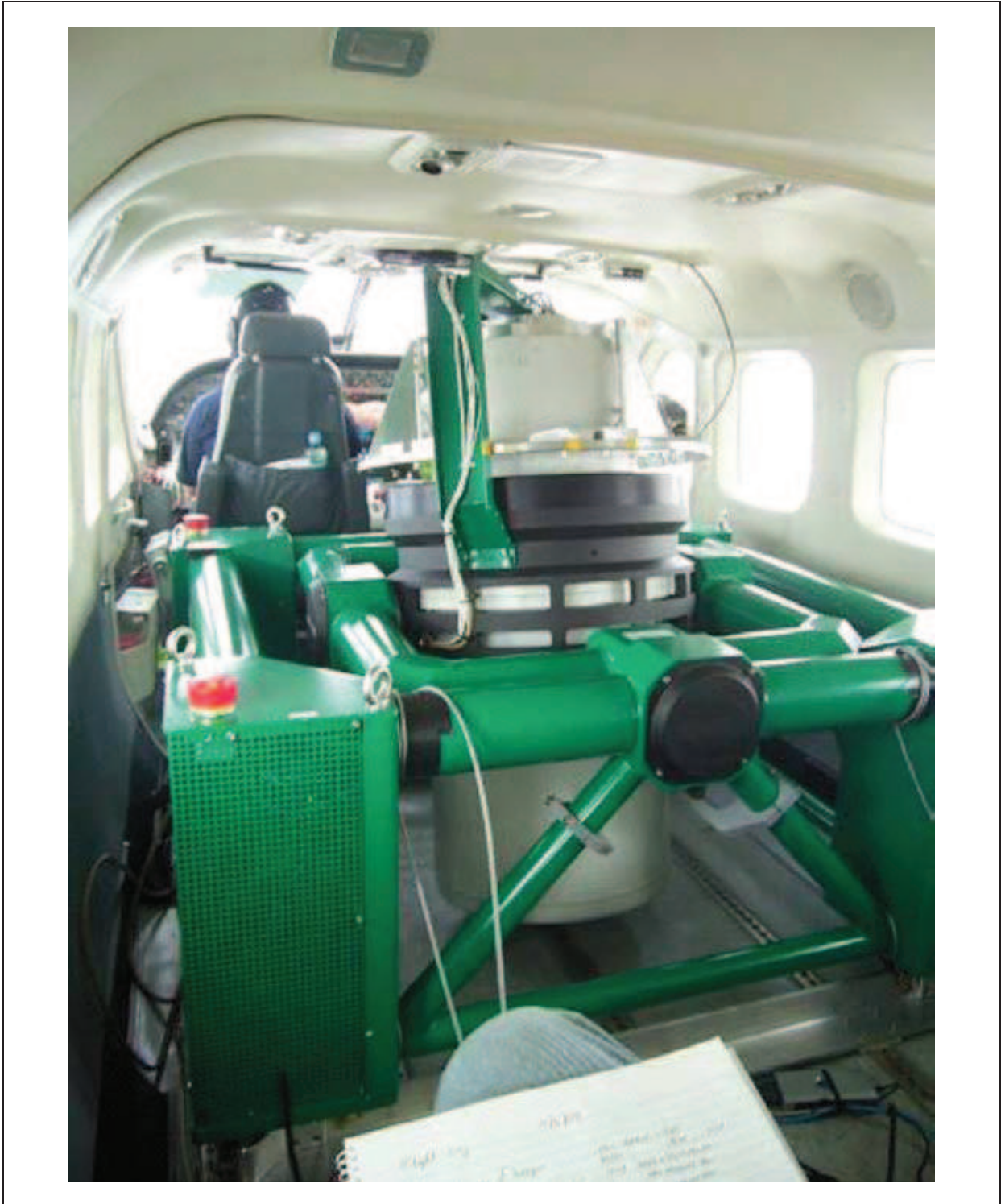
Figure 4. The rotational stabilisation platform, shown mounted in a Cessna 208. The platform (coloured green) stabilises the liquid helium dewar (grey cylinder), which houses the instrument. The instrument is operated in a vacuum inside a sealed chamber, which is immersed in liquid helium.
