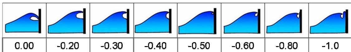
Figure 8 Wave shape before impact as a function of the focal point w.r.t. the wall.
