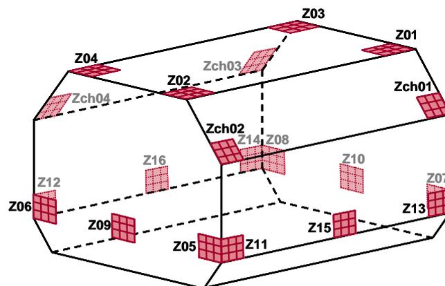
Figure 3 Small scale sloshing model tests (GTT) using hexapod and typical pressure sensors positions
