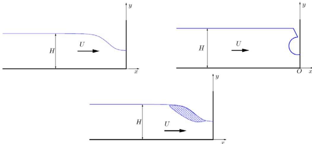
Figure 9 *Different impact types for low filling situation: steep wave, breaking wave and aerated*
