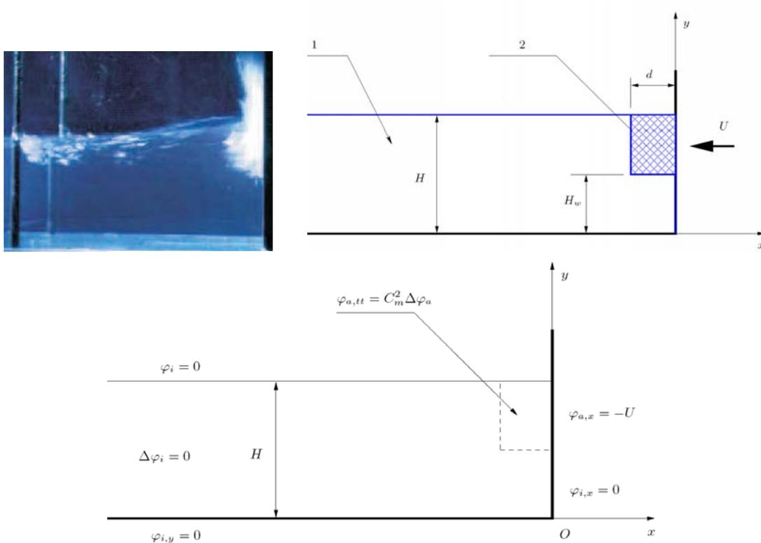
Figure 10 Aerated impact and corresponding simplification (Top –real situation and its geometrical simplification, Bottom – mathematical model)
