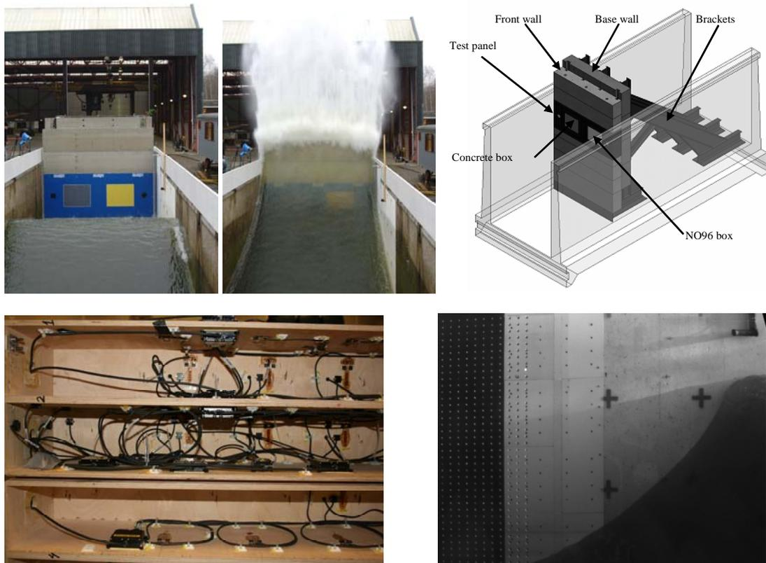
Figure 6 *Sloshe!* model tests (clockwise: wave flume, mounting scheme, iCAM sensor and instrumented NO96 box)
