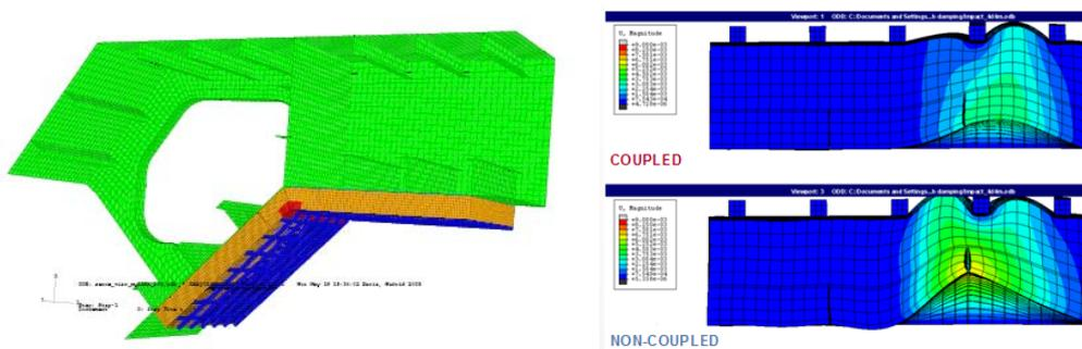
Figure 11 3DFEM structural model and comparison of the quasi static and hydroelastic structural responses
