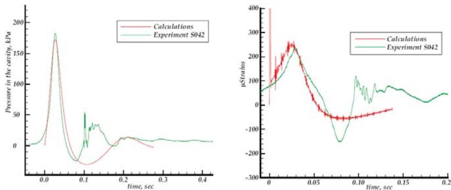
Figure 14 Pressure in the air pocket (left) and strain (right) in the cover plate during the breaking wave impact.
