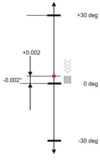
The corrective value for the nominal, maximum, negative inclination may now be entered. (According to the example -30°, displayed is -33°).
