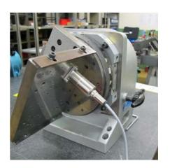
Copy the negative reading from the LEVELMETER 2000 on to paper. (e.g. -29.951°)
