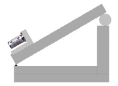
Copy the negative reading from the LEVELMETER 2000 on to paper. (E.g. -29.951°)
