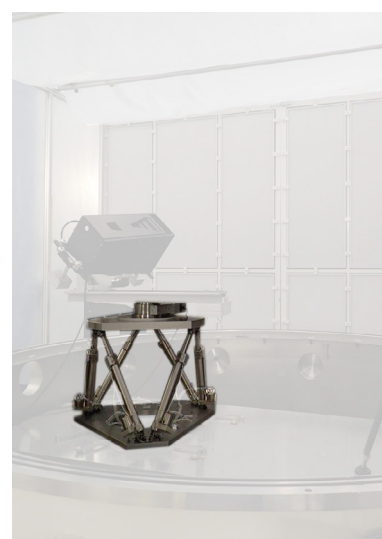
A vacuum compatible ZONDA hexapod is used at CSL to calibrate space optical instruments.
