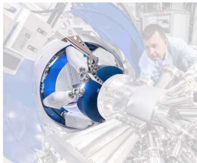
Diffractometer with BREVA hexapod on CEA BM32 beamline at ESRF synchrotron for the development and analysis of nanomaterials.
