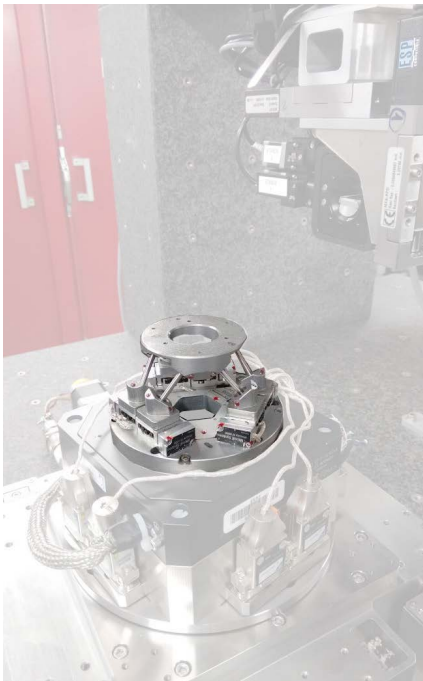
NanoPos hexapod is positioning a sample on ID11 new Nanoscope station of ESRF synchrotron. ID11 is a beamline dedicated to moderate to high energy diffraction and/or imaging studies of a variety of systems of interest for their physical, mechanical, or chemical properties.
